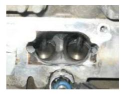
14. Check cleaning (with an endoscope if necessary). Repeat the procedure as often as needed to get a satisfactory result.
