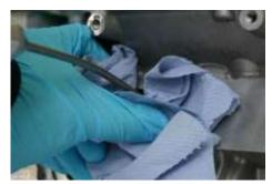
20. Cover intake ducting with a cloth and use the blow gun (4) to get rid of the neutralisation solution residue.
