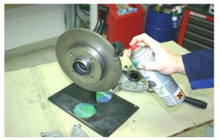
4. Apply MP 113 on the whole back side and the slide face of the brake pads.
