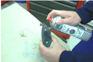
3. Clean the whole brake system. (brake calliper, calliper bracket)
