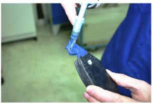
**5.** If the brake pad has a sticker on the back side, so you haven't to apply on the back, just on the slide face of the brake pad.
