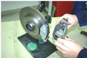
2. Clean the slide face and the back side of the brake pads.
